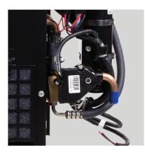
**Engine Waste Water Heat** Optional evaporater with heater core and water valve to provide vessel heating
